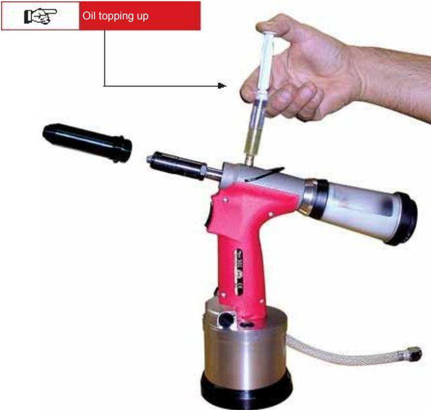
The topping up of the oil is necessary when occurs a power loss of the riveting tool or after a long period of use.
